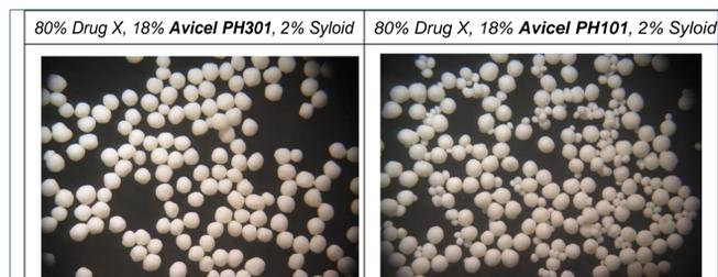
Figure 3: Microscopy images of core beads with different grades of Avicel.
