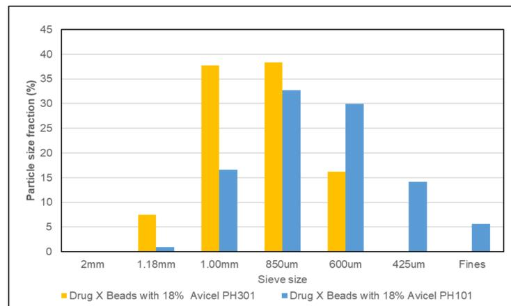
Figure 2: Particle size distribution comparison of formulation with Avicel PH101 and Avicel PH301
