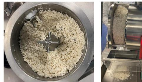
Figure 1: Wet mass end point (LHS), extrudate (RHS)
