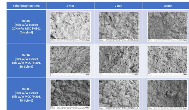
Figure 4: SEM images of the multiparticulates with increasing Syloid content from Top to Bottom and increasing spheronization time from Left to Right.
